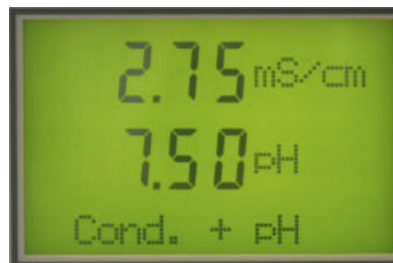
Simultaneous Conductivity and pH Measurement
